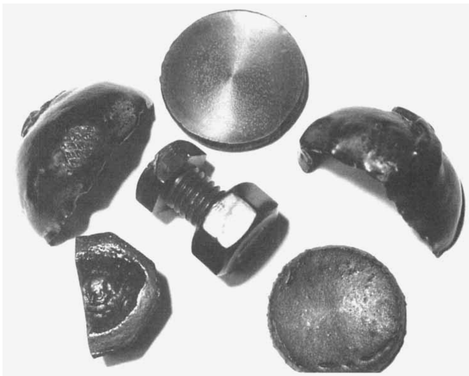
FIG. 5. First solid pieces of polychloral; initiator, lithium cholesteryl oxide; end-capped with phenylisocyanate.
